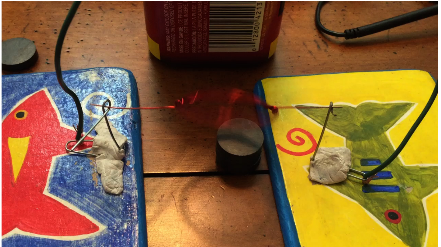
Figure 2: A Simple Motor.
