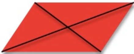
Figure 9: In a parallelogram, diagonals also bisect: each cuts the other into two line segments each of the same length.
